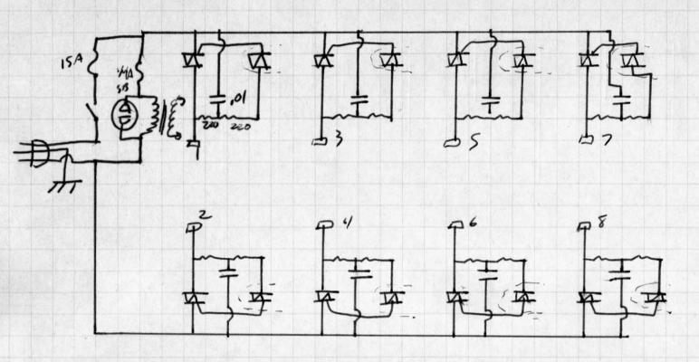
The R3AM and the R6M are a modification of the Standard R3A and R6 with an additional triac board included to allow MATRIX effects, also known as STARBURST eff-cts, where the lights will chase in pattern on 2 axis. Other than the changes shown above, and the inclusion of a matrix control board measuring 2" by 2" the units will have all the same components.
